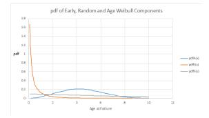
pdfA is the probability distribution function for age related failures as a function of the age of the component, pdfR for random failures and pdfE for early failures.
