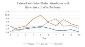
The plot is based on Lantz (2013).Generator and gearbox failure is not common when they are new, however it is not unusual for blades to fail when new. Note that blades do not seem to have a random failure component while generators and gearboxes do not seem to have an early component.
